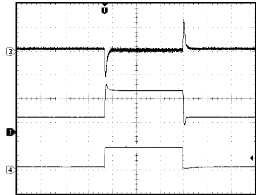
CH1 = COMP, CH3 = V_{OUT} , CH4 = I_{LOAD} (50mA TO 490mA) V_{IN} = 3.6V , V_{OUT} = 2.5V , C_{OUT} = 22\mu F , C_C = 150pF , R_C = 100k\Omega
